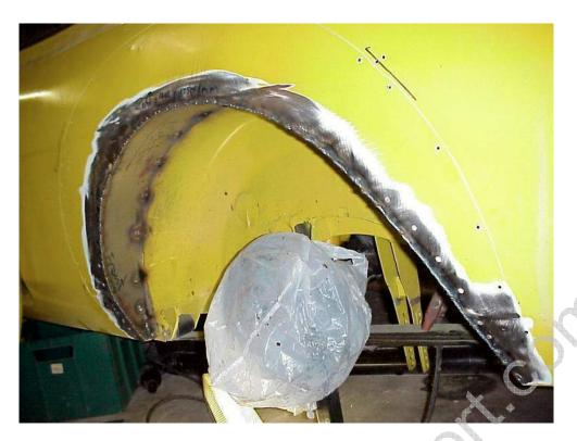
This is plug welded to existing wheel well and then joined to outer guard as shown.
