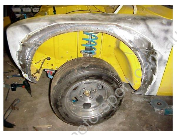
I slightly curved up the lip, of the metal guard edge, to conform with the fiberglass, for a better fit. Check to see that the bonding areas are touching and remove high spots with the sander, as required. Roughen up both surfaces with 36 grit paper. Fiberglass international, for example, have outlets in most states of OZ. Tell them you want to bond these fiberglass flares onto metal.
