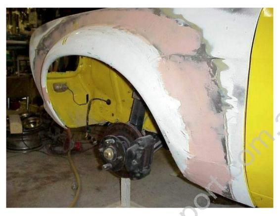
Under the guard needs to be as good as you want to make it. However it needs to be smooth and crevice free, to detract dirt/water ingress between the metal and fiberglass.
